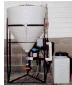
1Micro Bio Diesel Reactor
